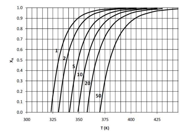
The inlet stream does not contain B and the concentration of A in the inlet stream is 5 mol/m³. The molar feed rate of A is 100 mol/s. A steady state energy balance for this CSTR results in the following relation:  $T = 350 + 25 X_A$  where T is the temperature (in K) of the exit stream and  $X_A$  is the conversion of A in the CSTR. For an exit conversion of 80% of A, the volume (in m³, rounded off to the first decimal place) of CSTR required is
