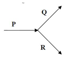
The flow rate of P, containing 30 mass% of ethanol, is 100 kg/h. What is the least number of additional specification (s) required to determine the mass flow rates and compositions (mass%) of the two exit steams?
