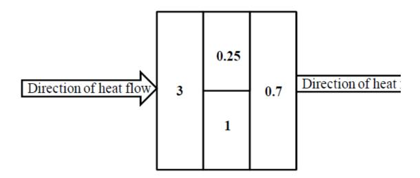
The overall resistance (in K/W, rounded off to the first decimal place) of the composite wall, in the direction of heat flow, is \_\_\_\_\_\_
